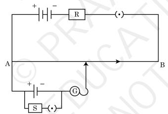
Keeping other things unchanged (a) X increases the value of resistance R, (b) Y decrease the value of resistance S in the set up. How will these changes affect the position of null point in each case and why?
