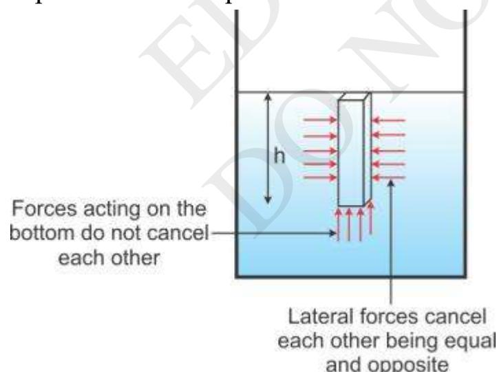
When a body is immersed in a liquid, the thrusts acting on the side walls of the body are neutralized as they are equal in magnitude and opposite in direction. However, the magnitudes of pressure on the
