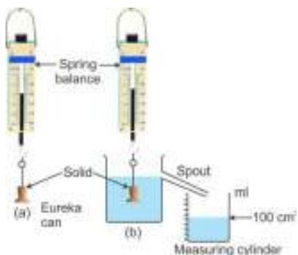
When the water stops dripping through the spout, note the weight of the solid and volume of water collected in the measuring cylinder.
