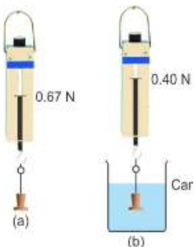
Take a solid body and suspend it by a thin thread from the hook of a spring balance as shown in the above figure (a). Note its weight. Above figure (a) shows the weight as 0.67 N.
